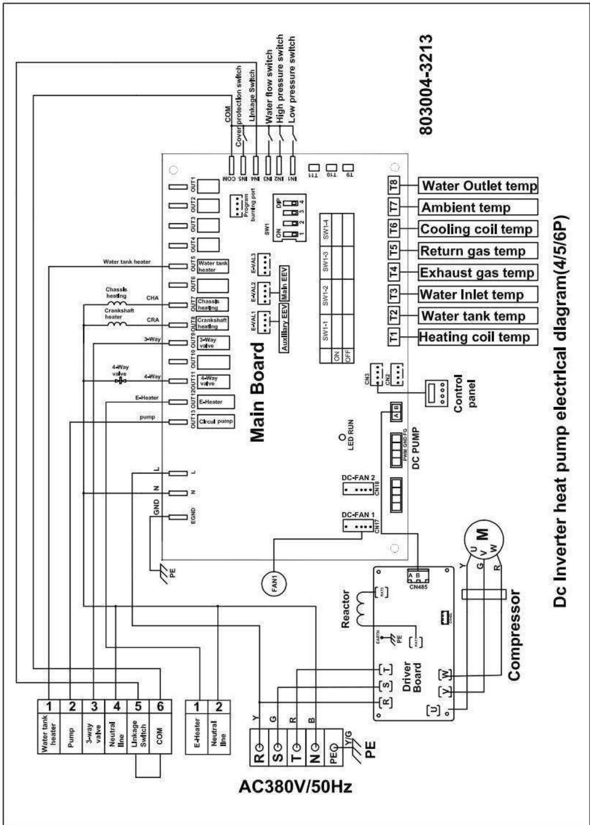
Dc Inverter heat pump electrical diagram(4/5/6P)
